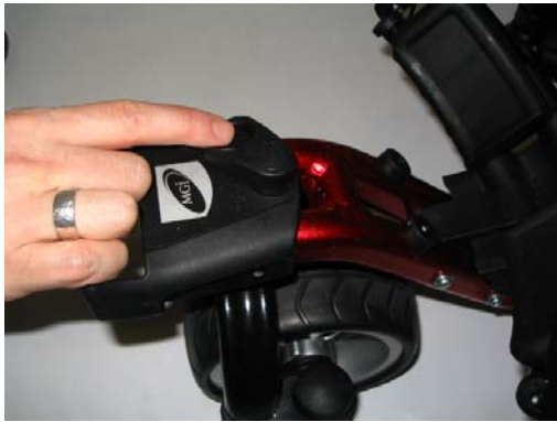
1. Move the lever to the left to unlock the front wheel assembly.
